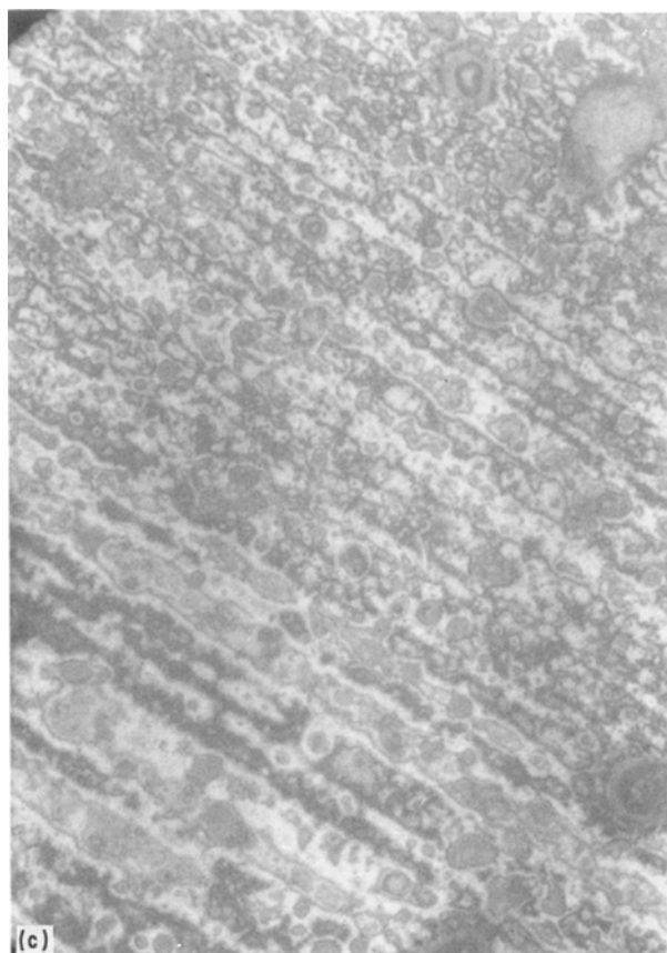
Figure 2 Reflection photomicrograph patterns taken for \text{Ag}_6(\text{As}_2\text{S}_3)_{94} film ( \approx 100 \mu\text{m} ) after isothermal annealing for different times at 200^\circ\text{C} : (a) 1 h, (b) 2 h, (c) 5 h. The film was prepared by ice-quenching from the melt. \times 315
