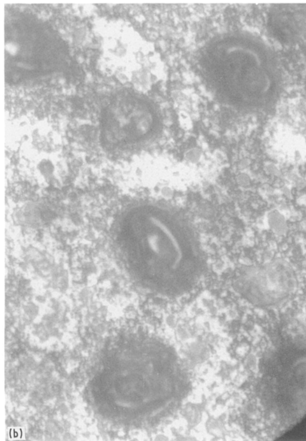
Figure 3 Reflection photomicrograph patterns taken for different Ag-As 2 S 3 films ( \approx 100 \mu\text{m} ) isothermally annealed at 200°C for 4 h: (a) Ag 6 (As 2 S 3 ) 94 , (b) Ag 15 (As 2 S 3 ) 85 , (c) Ag 25 (As 2 S 3 ) 75 . The films were prepared by ice-quenching from the melts. \times 315
